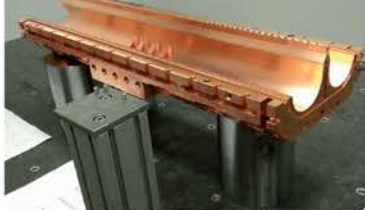
Acceleration structure used in the preliminary stages of the ion accelerators
